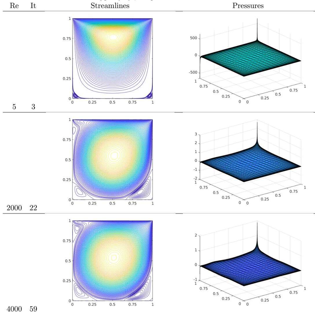
The maximum Reynolds we could compute with this parameters with the given script was 4837. We can see that new vortices appear when we increase the Reynolds number.
