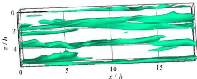
Streaky structures can be explained by a **linear local optimization**: two peaks in the energy gain curves varying the spanwise wave length [Pujals et al. 2009].
