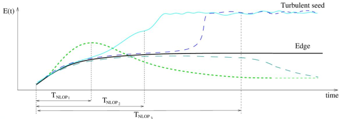
The **MINIMAL SEED** is the disturbance of minimal energy asymptotically approaching the edge state → its energy is the threshold energy for transition!
