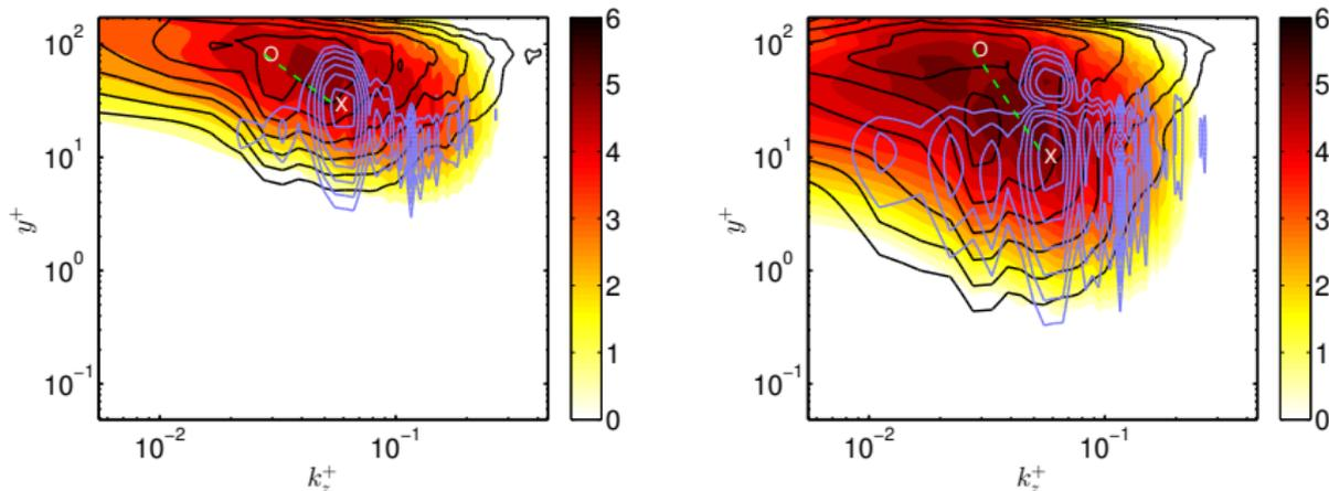
**Figure:** Logarithm of the premultiplied power energy spectra in the spanwise direction plotted as a function of the wall normal distance  $y^+$  (from left to right: wall-normal and spanwise velocity component).
