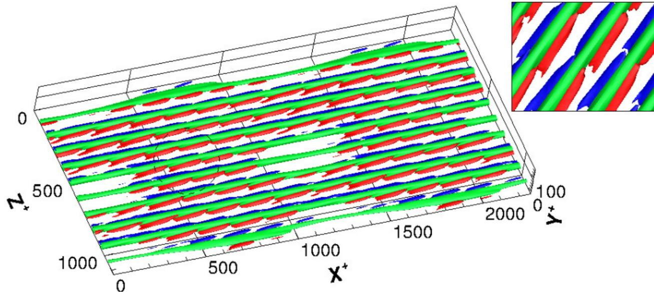
**Figure:** Shape of the optimal perturbation for  $T_{inner}$  and  $E_0 = 10^{-2}$ . Isosurface of the negative streamwise velocity (green) and Q-criterion coloured by contours of streamwise vorticity (positive blue, negative red).
