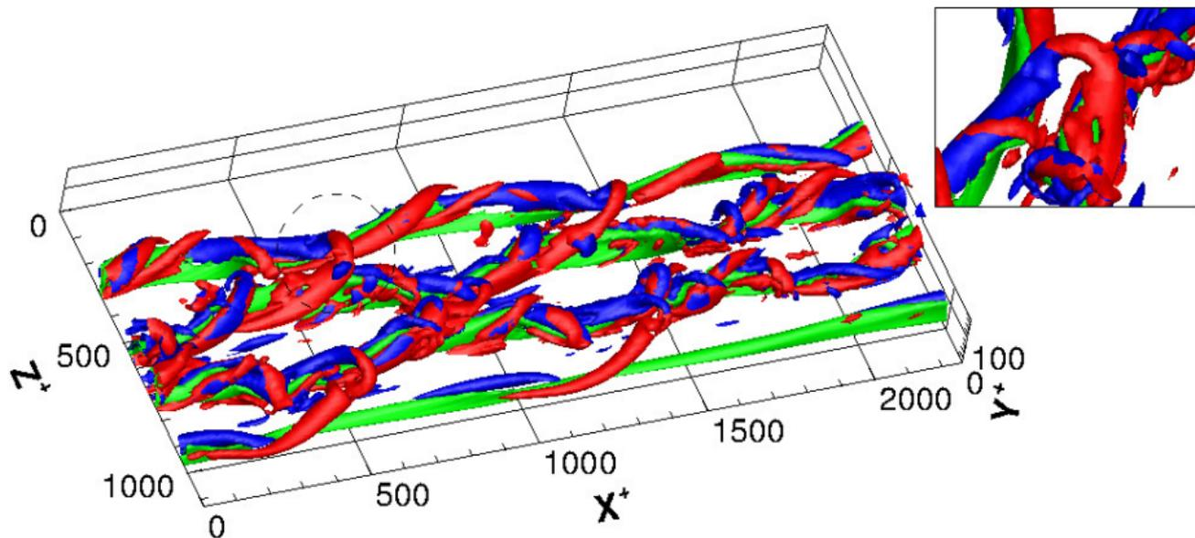
**Figure:** Shape of the optimal perturbation for  $T_{outer}$  and  $E_0 = 10^{-2}$ . Isosurface of the negative streamwise velocity (green) and Q-criterion coloured by contours of streamwise vorticity (positive blue, negative red).
