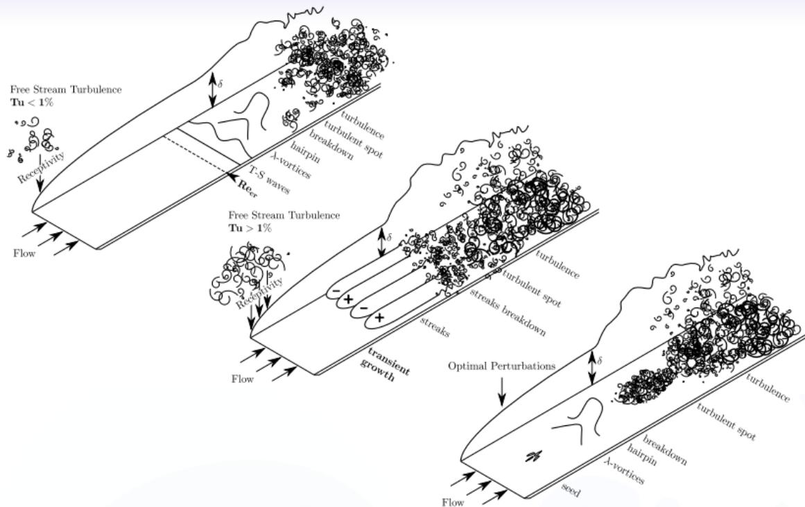
Transitional flow over a flat plate: (top) low-amplitude modal instability (middle) nonmodal linear instability (bottom) high-amplitude, nonlinear transition scenario
