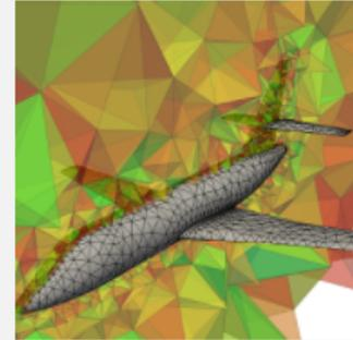
*Mesh for 3D Finite Element computations*
